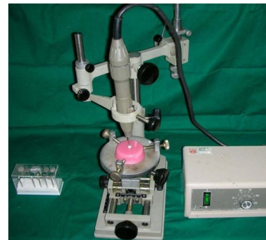
Figure 2: Ceramic samples on a mould base being polished on a surveyor
